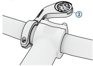
7 Press down slightly and turn the Edge bike computer clockwise until it locks into place.
